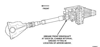
Front Driveshaft Grease Fitting
